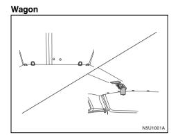
Top strap anchors are located at both sides of the floor mat in the rear cargo area behind the rear seat and at the center of the upper rear roof.
